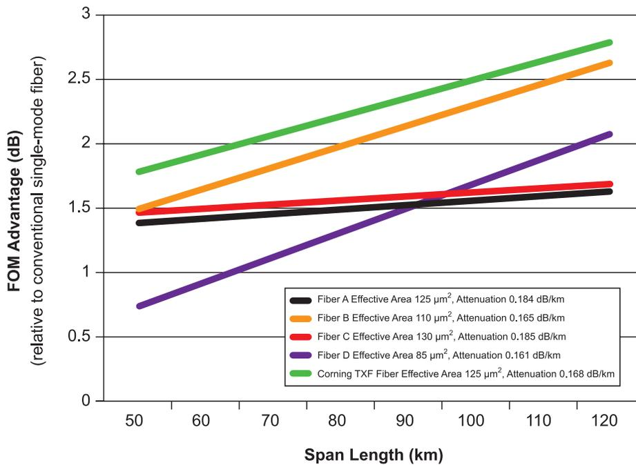
Figure 2. Corning TXF fiber performance advantage compared to other single-mode fiber designs targeted at terrestrial long-haul.
