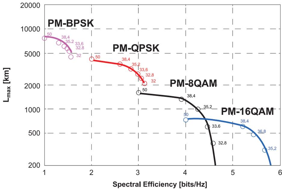
Figure 1. Impact on reach of upgrading to higher data rate protocols.
